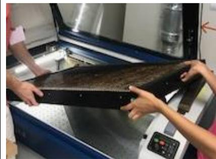
Now that everything is cleaned, carefully place the bed back into the laser machine and don't bang the carriage
