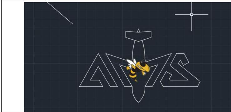
Delete box lines and material lines as well as anything within that area that should NOT be cut or rastered.
