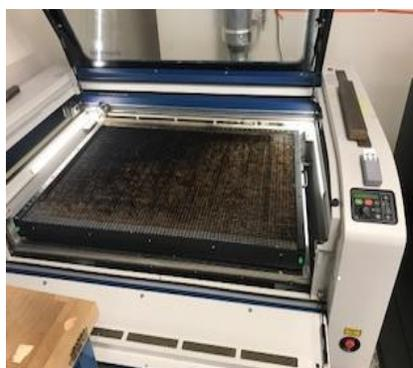
Make sure the alignment pegs on the laser bed fit into the alignment holes underneath. The bed should not be able to slide and look like it's back in place
