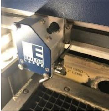
Put the carriage back in the laser and tighten (finger tight) the 3 screws. Note: The side rails must slide on top of the side pegs.
